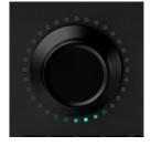
When Scroll mode is already activated, press the SCROLL button again to switch to Zoom mode. Two or more ring LEDs will light up in violet. Turn the Center Dial clockwise to zoom in horizontally, or counterclockwise to zoom out horizontally. The number of lit up LEDs will change depending on the current zoom level: the more you zoom out, the more LEDs will light up.
